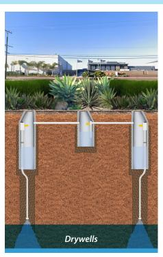
Drywells are an infiltration best management practice (BMP) designed to capture, treat and infiltrate stormwater runoff. They can also provide flood mitigation.
